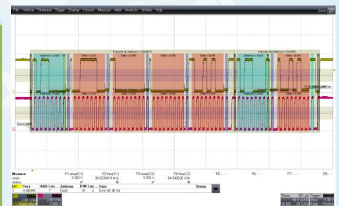
Fig. 5 Decode I 2 C-bus signal
